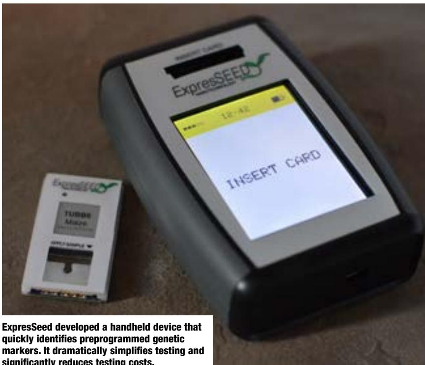
ExpresSeed developed a handheld device that quickly identifies preprogrammed genetic markers. It dramatically simplifies testing and significantly reduces testing costs.
